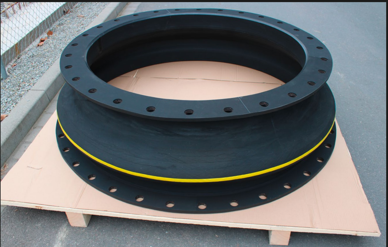
Single arch reducer made from NBR rubber with embedded vacuum ring, type U112A \varnothing 1,400 mm / \varnothing 1,200 mm, design pressure 5 bar
