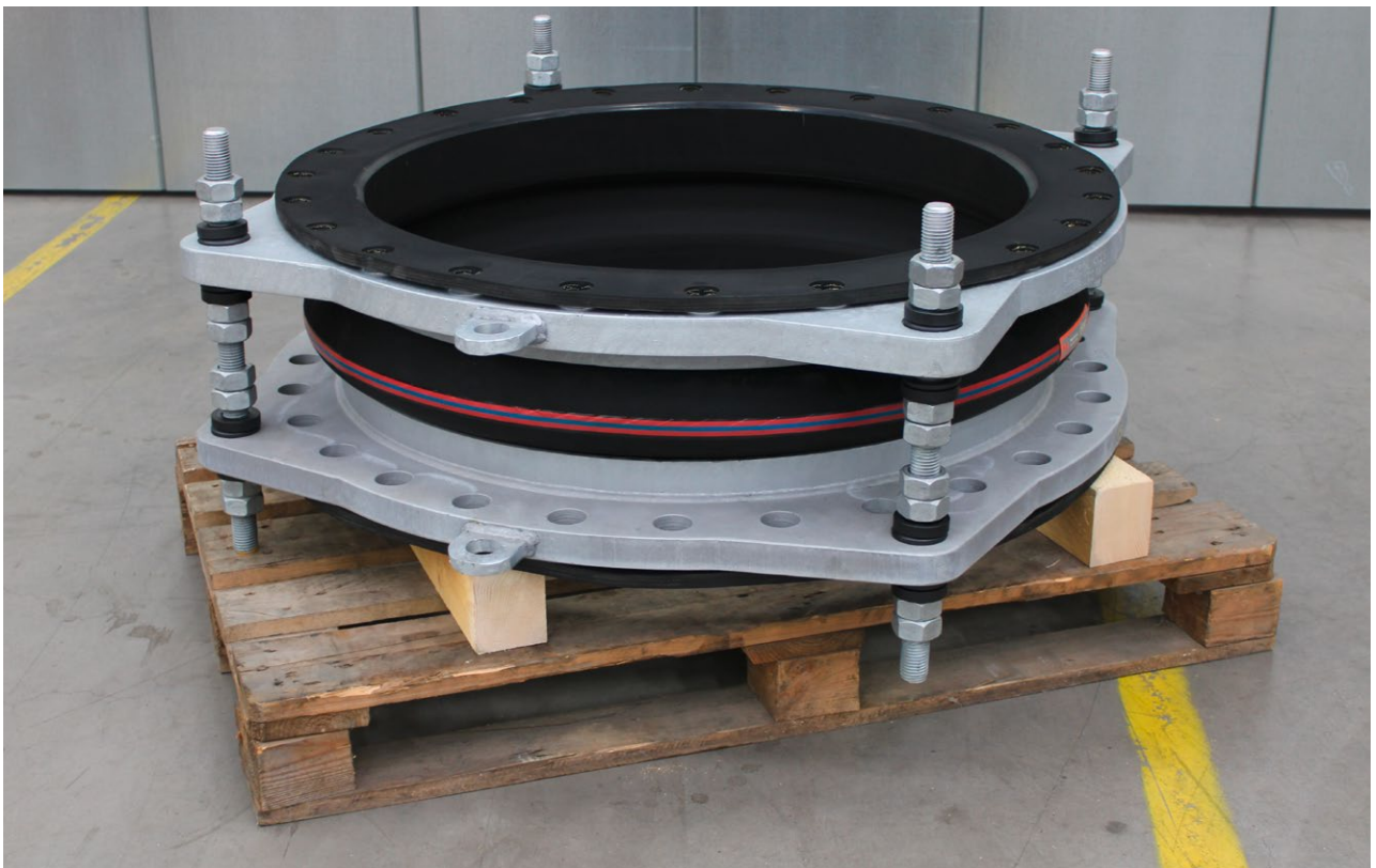
EPDM rubber expansion joint \varnothing 900 mm PN 16 designed according PED 2014/68/EU with aramid cord reinforcements, design temperature 120° C
