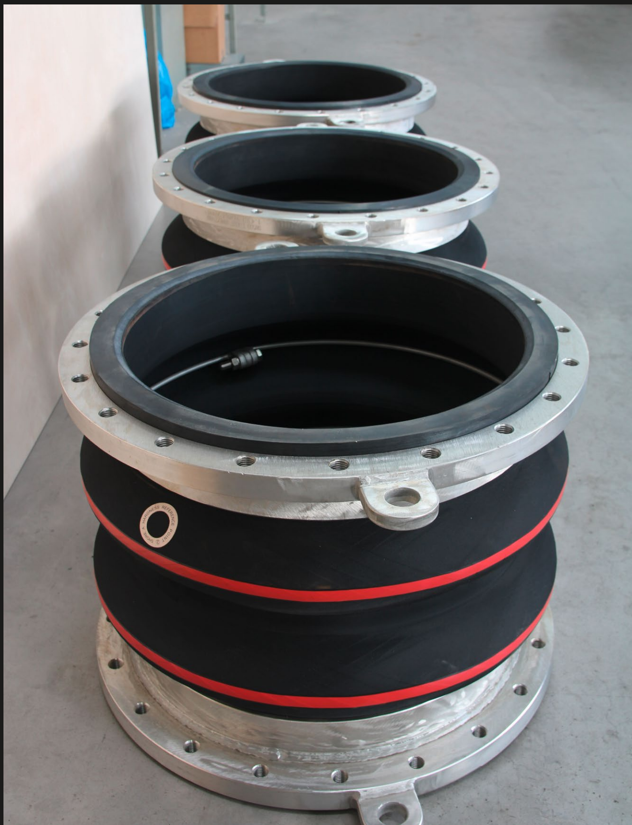
Double arch EPDM rubber expansion joints \varnothing 500 mm with stainless steel swivel flanges, for permanent vacuum operation in a paper mill
