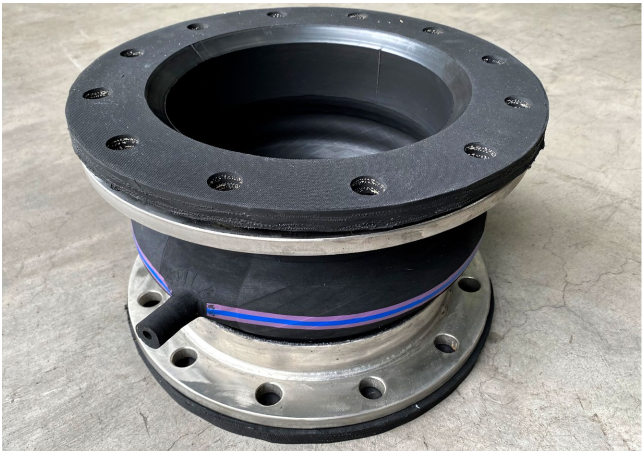
Homogen vulcanized two ply testable rubber bellows of size \varnothing 300 mm made from FPM rubber for a chemical plant
